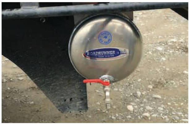
Under deck mounted Water Tank WT-02.
