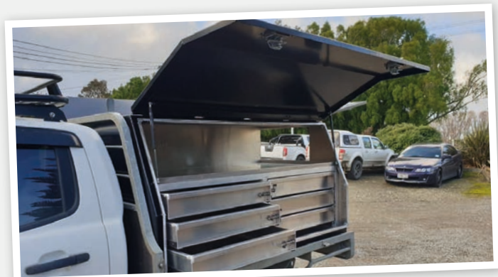
Service Box with pull out draws.
